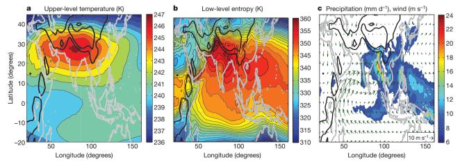
Figure 1 | Observational estimates of June–August thermodynamic structure, precipitation and wind. a, Satellite-based (AIRS) estimate of mass-weighted vertical mean temperature for  $175-450\,\mathrm{hPa}$ . b, ERA40 equivalent potential temperature on a terrain-following model level about
